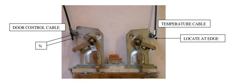
SHORTEST of the cables is the door control cable. Lay control assembly on the bench as shown in the picture above. Attach this cable to left control lever using the original cable clip, screw and push nut. Cable housing is located 3/4" past edge of the bracket.
