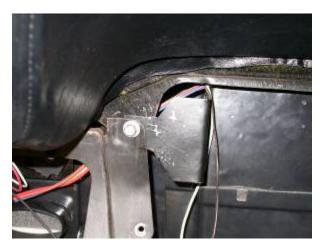
Loosely attach front evaporator mounting bracket through center mounting plate and into dash using (1) of the original bolts.
