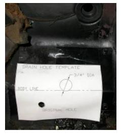
Locate the drain tube template on last page of the instructions.
