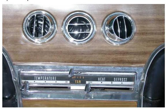
THE PICTURE YOU SEE ABOVE SHOWS THE CONTROLS IN THE A/C MODE. THIS MEANS THAT THE AIR WILL BE DISTRIBUTED THROUGH THE FACE OUTLETS. THIS ALSO HAS THE TEMPERATURE LEVER IN THE COLD POSITION. WITH THE CONTROLS IN THIS POSITION YOU WILL GET THE AIR THROUGH THE FACE OUTLETS AT THE COLDEST TEMPERATURE.
