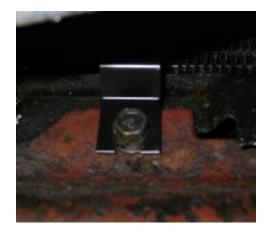
Locate left bottom condenser mounting bracket and slide into the bottom radiator mounting bolt.
