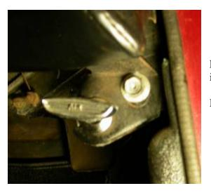
Located on passenger side, on bottom of the dash cover pad is the fresh air door cable.
