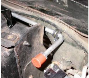
Locate (1) 3/8" tube clamp and (1) #10 x 3/4" tek screw.
