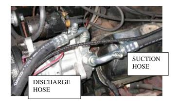
Locate #8 discharge hose and (2) #8 o-ring. Attach end of hose with 45 deg fitting to the condenser fitting and the end with the service port to the compressor.
