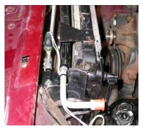
Slide condenser between radiator and the radiator bulkhead. Let condenser hange on the upper brackets.
