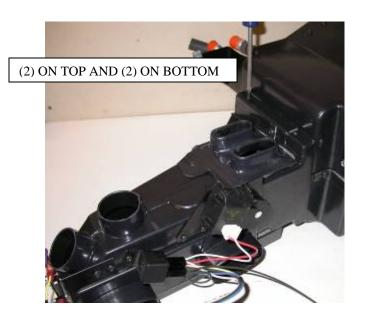
Locate the evaporator, Air Distribution Duct assembly and (4) #10 x 5/8" pan head screws.
