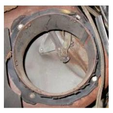
Locate air inlet flange assembly directly above the passenger kick panel.
