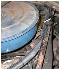
When routing suction hose tywrap the hose to the body brace beside the air cleaner.
