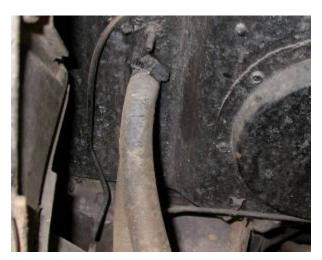
Drain radiator. Disconnect heater hoses at the firewall.
