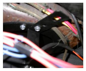
Attach mounting bracket on the blower to edge of the air inlet block off using (1)  $\#10 \times 3\%$ " tek screw.
