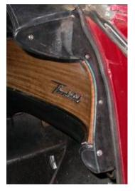
Located on passenger side of the dash is a trim plate, remove and retain trim plate and hardware.
