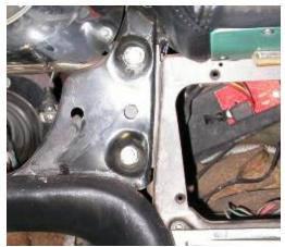
Remove (2) mounting bolts on drivers side of the center mounting plate.
