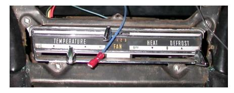
Remove (4) screws holding the control head to the center mounting plate.
