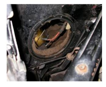
CAREFULLY REMOVE HEATER ASSEMBLY FROM UNDER THE DASH. DISCARD HEATER ASSEMBLY.
