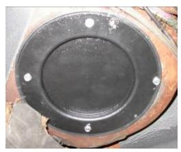
Locate the firewall block off plate.
