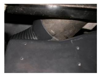
Route short defrost flex hose over top of the evaporator and push over the defrost diffuser.
