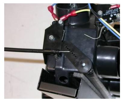
Route the longest of the control cables across back of the evaporator and out through grommet in the firewall block off.
