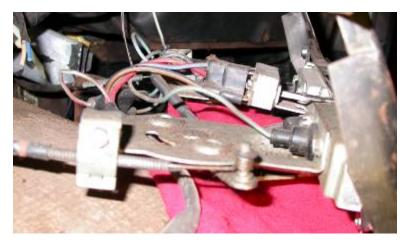
Disconnect control cables on both sides of the control head. Retain screws and the clips.
