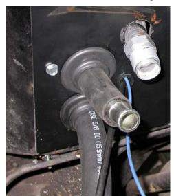
Attach water valve to lower hose from the evaporator using (2) worm gear clamps. Other end of water valve attaches to the return line to the motor.
