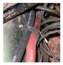
When routing liquid hose attach hose and the return heater hose to the shock tower using (1) double clamp and a #10 tek screw.
