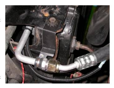
Locate (2) white wires tywraped to the discharge tube. Route along the discharge hose. Cut one of the wires and attach female bullet connector provided and plug into the compressor clutch wire.
